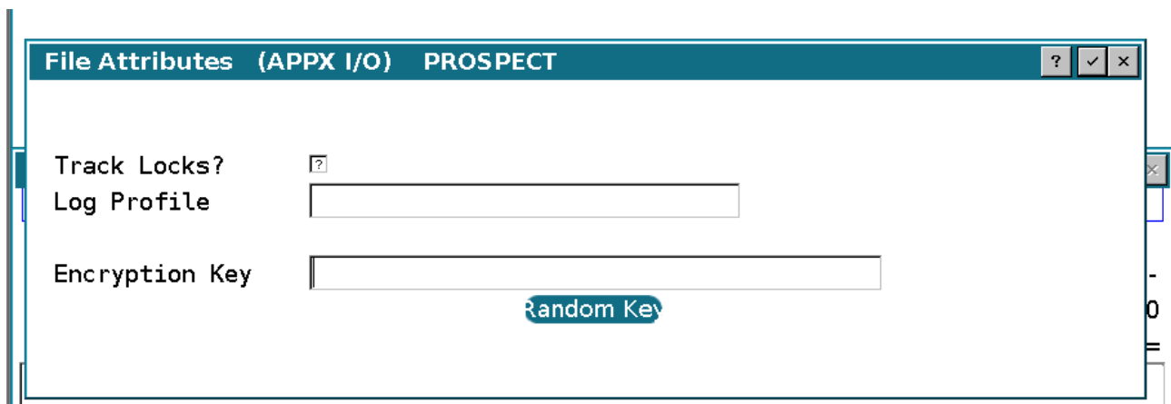
Figure 7. PROSPECT's file key cleared after export. The physical file is still encrypted until the replacement import.
